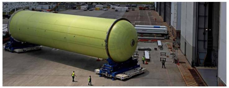
MAF\_20210429\_CS2\_LH2toVAB579: This image highlights the liquid hydrogen tank that will be used on the core stage of NASA's Space Launch System rocket for Artemis II, the first crewed mission of NASA's Artemis program. The tank is being built at NASA's Michoud Assembly Facility in New Orleans.
